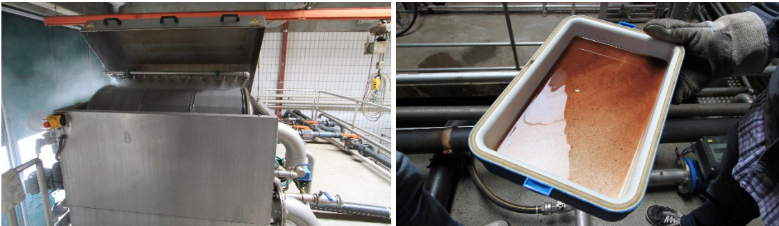
Figure 5-6: DEMON® Process - granule retention screen (left), granules sample (right)
